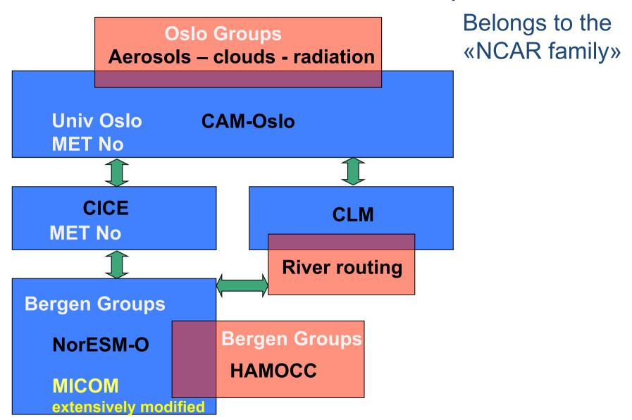
Components in blue communicate trough the coupler CPL7. Components in red are subroutines of blue components.
