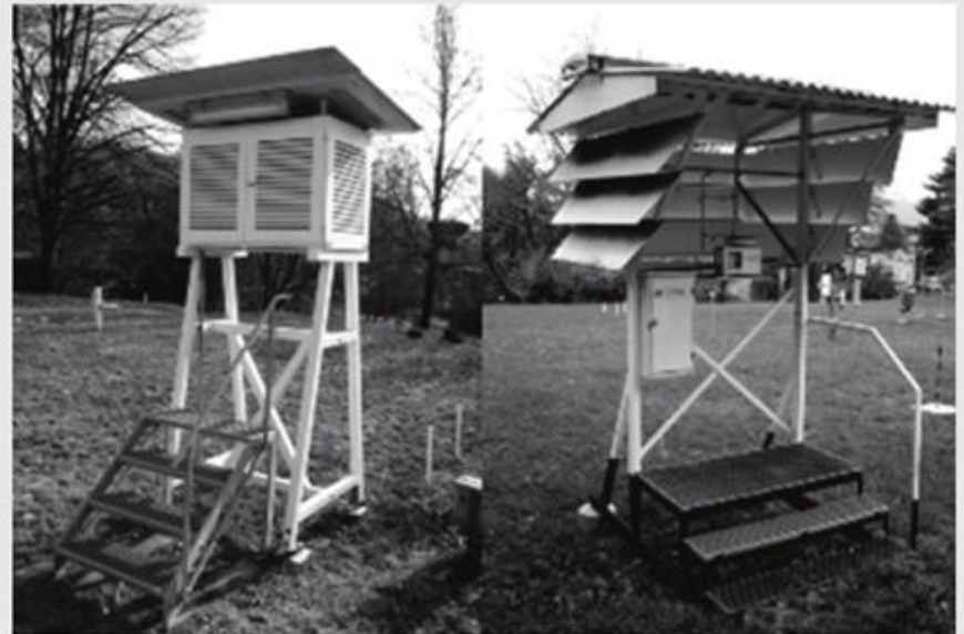
A standard Stevenson screen and a historical French screen measuring in parallel at an observatory in Basel, Switzerland.
