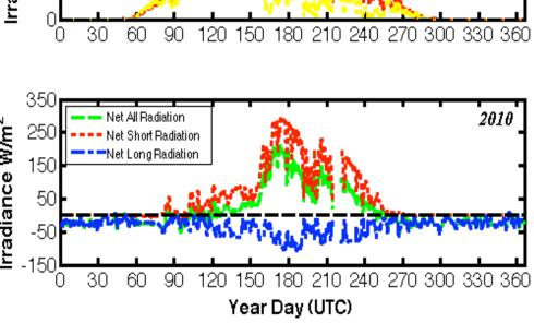
Annual cycles of daily averaged SW radiation (Kipp&Zonen CM22) and calculated net radiative energy, measured at the Eureka Flux. LW radiation component was measured by Eppley PIR
