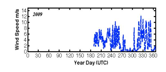
Annual cycles of daily averaged air temperature, measured at 2, 6, 10 m at the Eureka Flux Tower by Type-E Thermocouple/Campbell ASPTC-L and wind speed, measured at 10.5 m by RM Young Sentry anemometer
