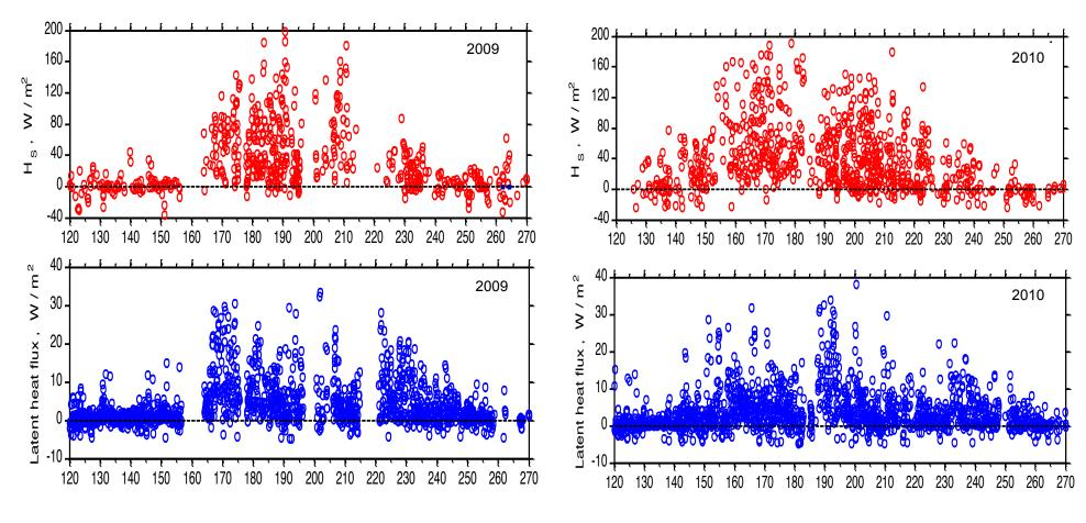
May-September time series of the hourly averaged sensible heat flux ( $H_s$ ), and latent heat flux ( $H_l$ ,). Measurements were made by sonic anemometers located at 3 and 8 m, and Licor-7500 at 8m.
