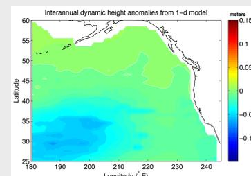
**Figure 6:** Simulated interannual steric height variability from model. These changes are due solely to thermal expansion.
