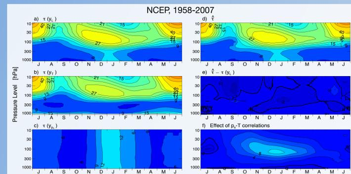
Left panels show the seasonality of the NAM time scale calculated for the a) linearized geopotential, b) temperature component and c) surface pressure component. Right panels show d) effective timescale estimate (see below) e) difference of d-a and f) cross correlation timescale due to  $T$ - $p_s$  correlations.
