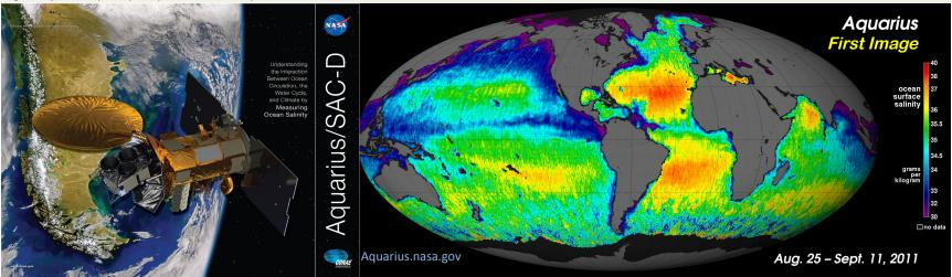
Figure 1 (Above Left): The Aquarius/SAC-D Satellite artist's conception in orbit over Patagonia. The satellite is in a polar sun-synchronous (6pm/6am) orbit that provides global coverage every 7 days.
