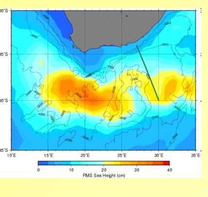
**Left**: root-mean-square (rms) of sea height over the Agulhas Current retroflection region between November 1992 and December 2004. The bathymetry contours are superimposed. The time-series of geostrophic transport of the Agulhas Current is estimated across a selected transect (green line).
