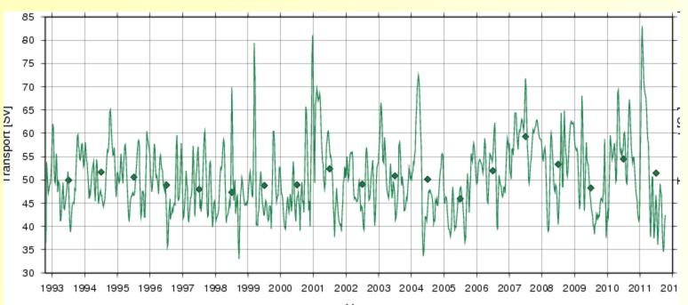
Above: time series of geostrophic transport of the Agulhas Current is produced using a combination of sea height anomaly (SHA) fields from satellite altimetry (AVISO) and climatological data (Levitus). Diamonds indicate the annual mean values.
