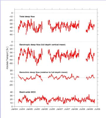
**Figure 1:** Deep transport in the western basin (800 to 4800 dbars) integrated from the shelf to the Mid Atlantic Ridge, plotted as the total transport, the barotropic transport (defined based on a full-depth vertical average), and the baroclinic transport (defined as the difference from the full-depth vertical average). Also shown is the basin-wide MOC upper-ocean transport from the basin-wide array. (From Meinen *et al.*, 2011)
