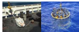
Above: A pressure-equipped inverted echo sounder (left) being prepared for deployment, and (right) a CTD being lowered; both are used for measuring the Deep Western Boundary Current.
