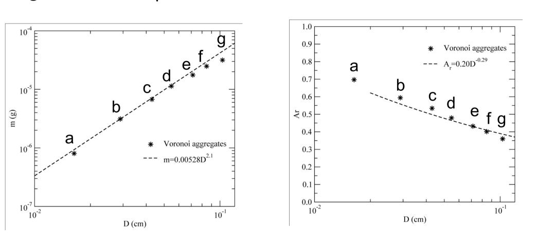
The models of irregularly shaped particles have fractal-like shapes, which is consistent with the measured m-D and Ar-D relationships. Moreover, the modeled particles have irregular structure not only in their overall shapes, but also in each cell of the particle elements.
