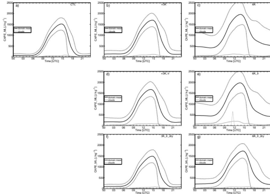
**Figure 4.4:** Mean diurnal cycle of CAPE ( $\text{J kg}^{-1}$ ) with domain mean values in black and cloudy points in grey for (a) CTL, (b) 3K, (c) 6K, (d) 3K\_Ir, (e) 6K\_Ir, (f) 3K\_Ir\_dry and (g) 6K\_Ir\_dry. Mean values are shown by the solid lines while the 10th and 90th percentile are shown by the dashed lines. The 10th and 90th percentile were calculated by considering all grid points on all 15 days.
