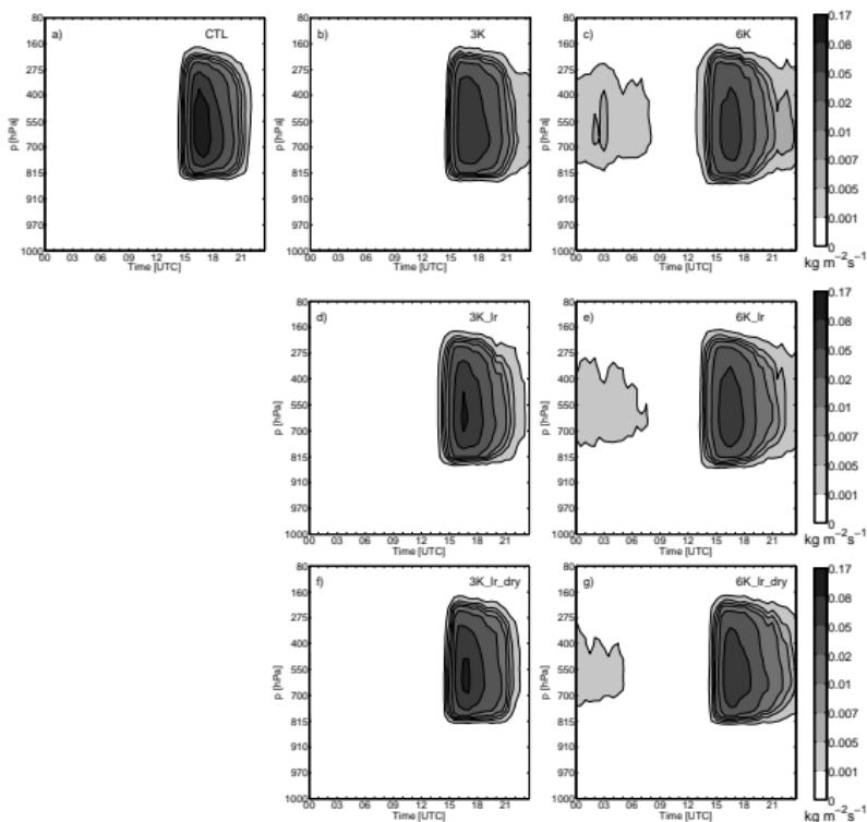
**Figure 4.5:** Mean diurnal cycle of convective mass-flux ( $\text{kg m}^{-2} \text{s}^{-1}$ ) for the set of simulations.
