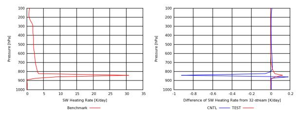
Figure 1: Calculated shortwave heating rate profile in the SCM (unit: K/day). Left: benchmark results; right: differences in CNTL (blue line) and TEST (red line) from the benchmark
