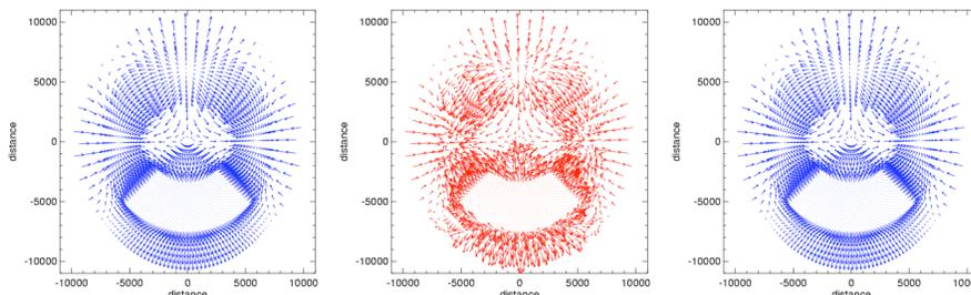
**Figure 2:** A large-scale divergent wind field (left panel) is perturbed by a small-scale rotational wind field (middle panel). The convolution filter is applied outside the uniform high resolution region and the filtered field is represented in the right panel.
