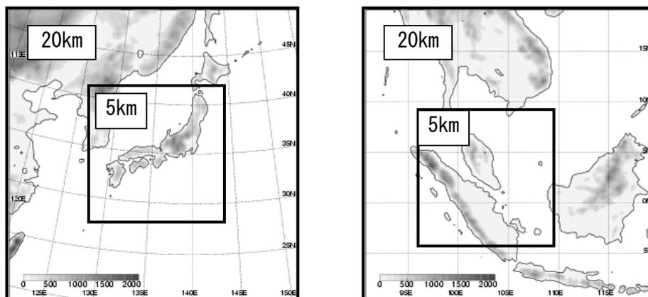
Fig. 1 Model domain and topography for Japan region and Southeast Asian region, with 20km horizontal resolution and 160 x 160 grid (3200 km square), with 5km horizontal resolution and 301 x 301 grid (1500 km square).
