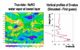
Fig. 6 (left) Difference between the true data and the assimilated fields of conventional data. (right) Vertical profile of difference of the true data and first guess data
