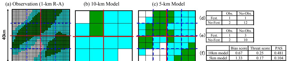
Fig.2. Schematic diagrams to compare the threat and bias scores with PAS, contingency tables, and verification results.
