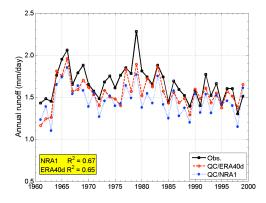
Fig. 1. Mean annual runoff over the 10-basin composite from two CRCM/CLASS simulations performed over the small QC domain, one being driven by NRA1 (dots) and the other by ERA40 (dash); continuous line shows observations.
