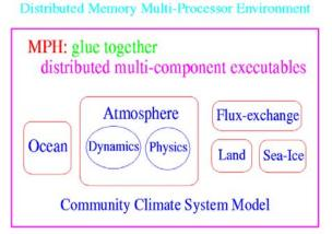
these component models are loaded into different set of processors; however, each model does not know the other models, their names, their processor-allocations, etc. A critical task on such distributed memory multi-component computer is a handshaking process that enables every component models to get the necessary information about other component models.
