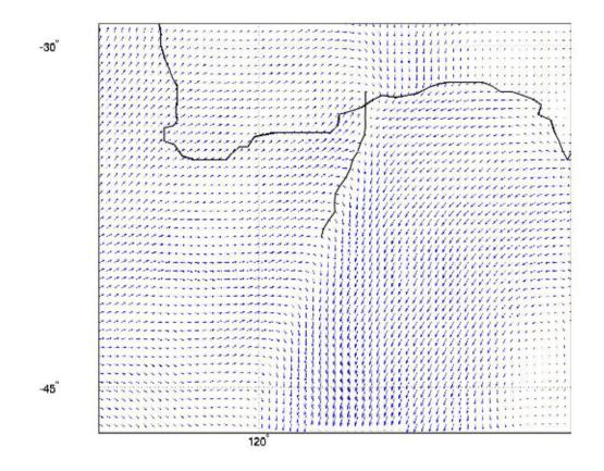
**Figure 1:** An example of a very preliminary version of the frontal identification scheme applied to the surface wind field of an arbitrarily chosen (29/12/2000 at 500 UTC) 6-hour forecast of the ALAPS model (Adams, 2004) run at 0.375° lat-long. resolution.
