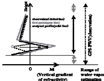
Fig.1 Schematic illustration how to determine the sign of vertical gradient of refractivity
