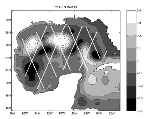
**Figure 1.** The sea surface height from the COAPS/FSU Gulf of Mexico numerical simulation using the Navy Coastal Ocean Model (NCOM). The white lines are simulated Topex/Poseidon tracks.
