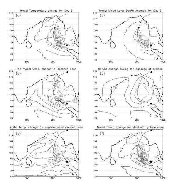
Fig1 : Model mixed layer depth anomaly and temperature change compared with observed SST change and temp. change in superimposed cyclone case. Solid line indicates the storm track.
