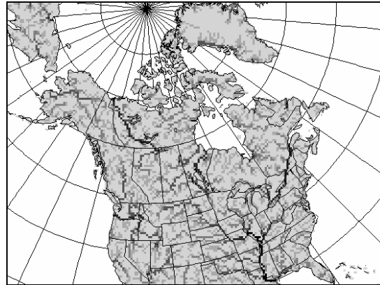
Figure 4: River order, which varies between 1 and 6 in this case, for the digital river networks obtained at the CRCM resolution.
