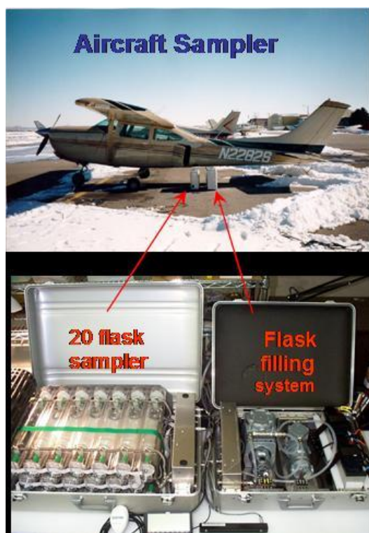
Figure 1: NOAA installation for sampling vertical profiles.
