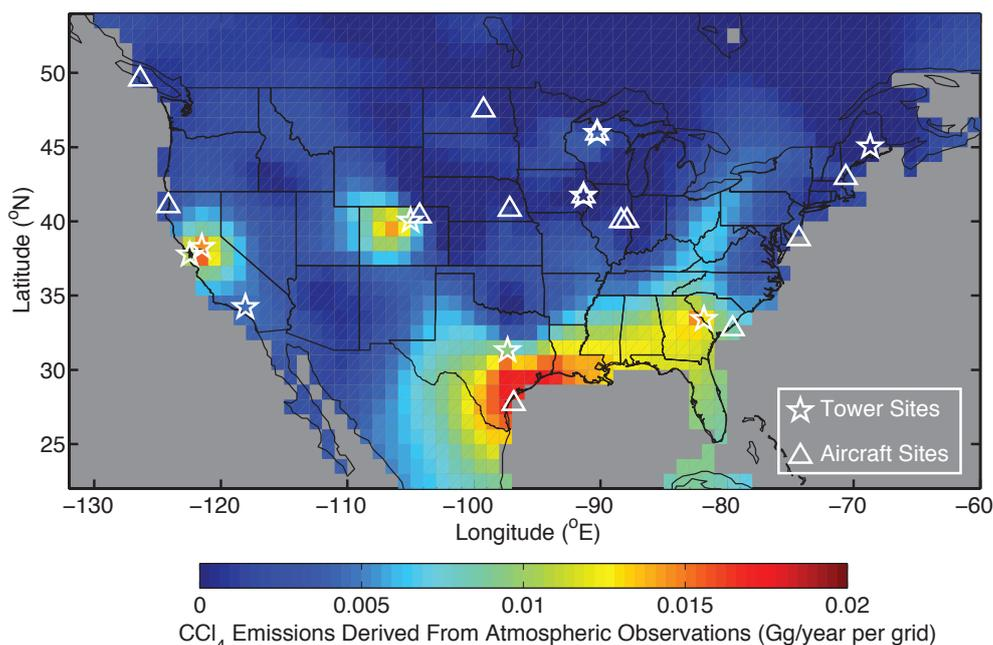
**Figure 10:** Spatially resolved  $\text{CCl}_4$  emissions over the U.S. derived from atmospheric observations during 2008-2012. The derived emission rate is indicated by the colour scale; the total mean emissions during this period were 4 (2-6.5) Gg/year. Emissions were derived from ongoing NOAA flask measurements from towers or aircraft at locations indicated by the symbols. Adapted from Hu *et al.* [2016].
