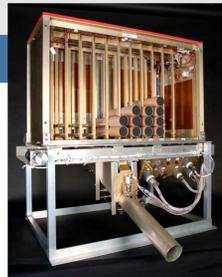
Dropsonde System designed and built by NCAR for NOAA to use on the NASA Global Hawk Unmanned Aircraft System. Capacity: 88 sondes
