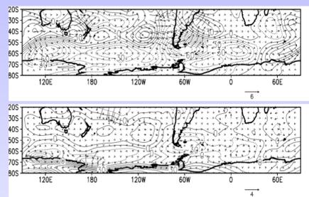
GPH zonal asymmetries (streamfunction temporal anomalies minus streamfunction zonal average) for 2010 singularly-cold summer at 300hPa (top) and 850hPa (bottom), and associated horizontal component of the wave-activity flux (vectors). Dashed contours correspond to negative GPH zonal asymmetries. The contour interval is 10 m. Vector units are m<sup>2</sup> s<sup>-2</sup>.
