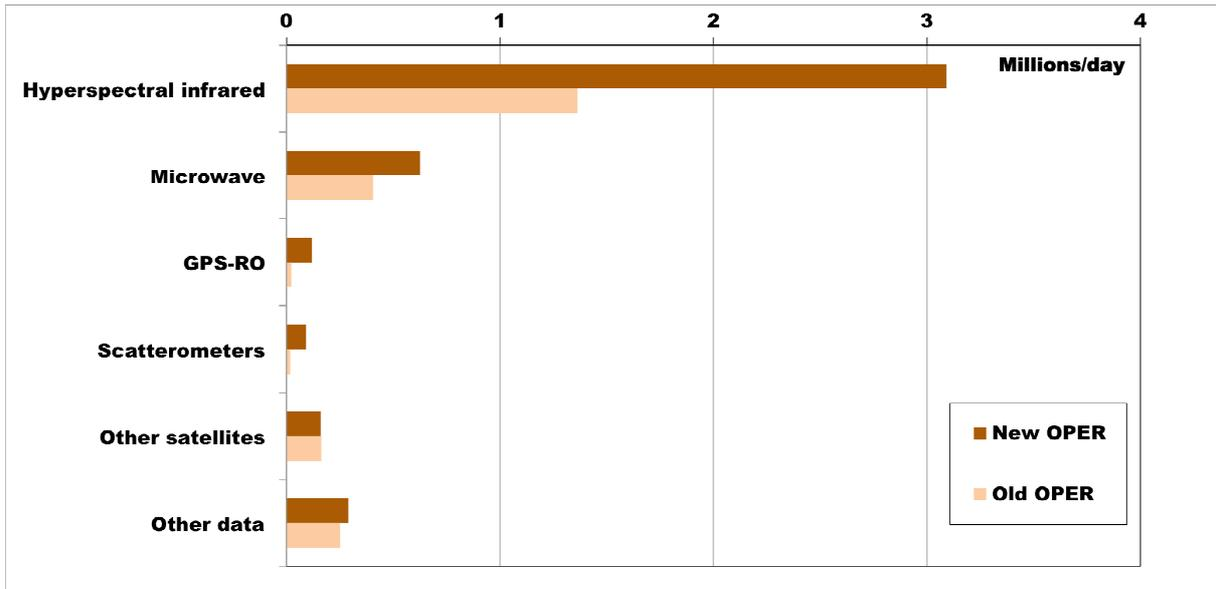
**Figure 1 :** Comparison of daily observations assimilated in the global model ARPEGE for the main observing systems (instruments onboard satellites: hyperspectral infrared sounders, microwave sounders and imagers, temperature measurements from GPS radio-occultation, surface wind measurements from scatterometers; other satellite observations; other data from radiosoundings, surface networks, aircrafts, and buoys) since the 02 July 2013 (**New OPER**) and before this date (**Old OPER**).
