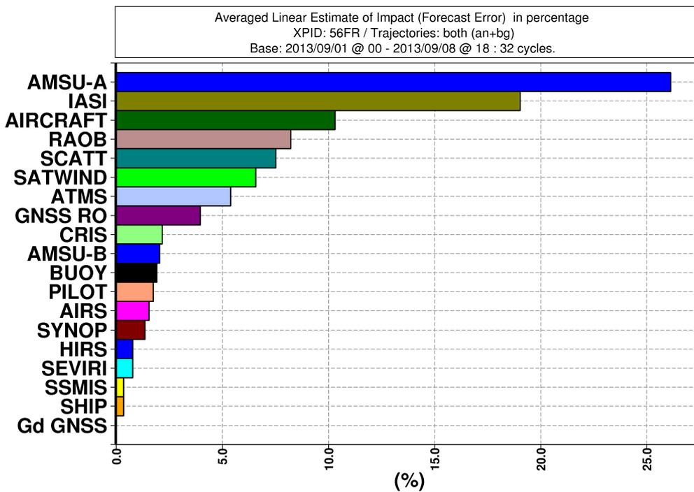
**Figure 2 :** Percentage of reduction in 24-h forecast errors (dry energy norm) in the Météo-France global model ARPEGE with the **new OPER** system (since 02 July 2013) resulting from the use of various observation types as diagnosed by the adjoint method.
