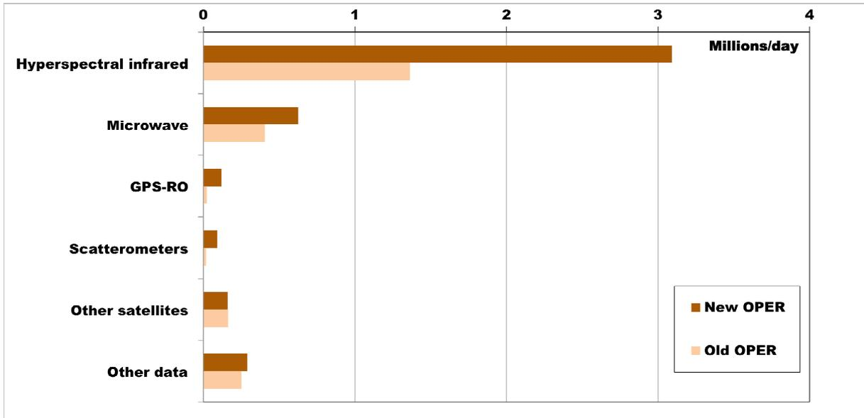
**Figure 1 :** Comparison of daily observations assimilated in the global model ARPEGE for the main observing systems (instruments onboard satellites: hyperspectral infrared sounders, microwave sounders and imagers, temperature measurements from GPS radio-occultation, surface wind measurements from scatterometers; other satellite observations; other data from radiosoundings, surface networks, aircrafts, and buoys) since the 02 July 2013 (**New OPER**) and before this date (**Old OPER**).
