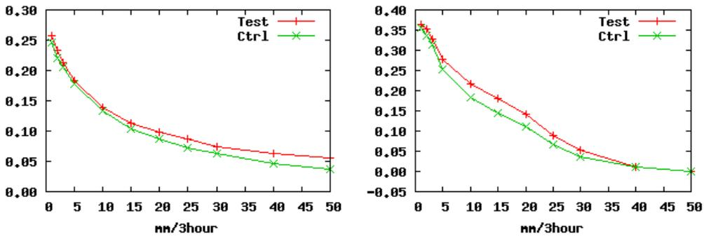
Fig. 1: Equitable threat scores of three-hourly accumulated precipitation forecasts in summer (right) and winter (left). The red and green lines show the results of JNoVA (Test) and Meso 4D-Var (CTRL), respectively. The horizontal axis is the threshold value of the rainfall amount.
