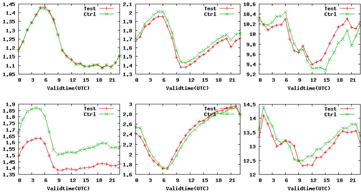
Fig. 2: Root mean square errors of wind velocity, temperature and relative humidity at the surface are shown from left to right, respectively. The upper panels are the results for summer, and the lower ones are those for winter. The line colors are the same as those in Fig. 1. The horizontal axis is the valid time, which is the real time of the forecast.
