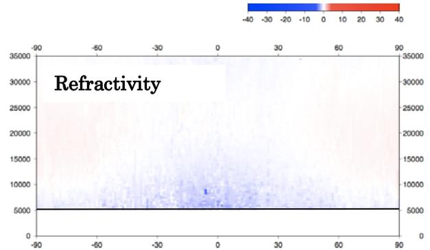
Fig.2 Amount of bias correction of refractivity. The data were used with height from 5km to 35km.
