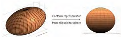
Figure A1-1: passage from the ellipsoid (\varphi, \lambda) to the sphere (\Phi, \Lambda) (Gauss–Laborde transformation)
