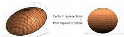
Figure A1-4: passage from the ellipsoid (\varphi, \lambda) to the sphere (\Phi, \Lambda)
